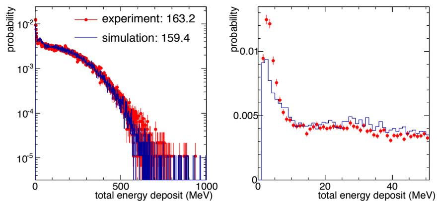
**Figure 6.** Total energy deposited in the NeuLAND prototype. Points - experimental data, histogram - simulation.
