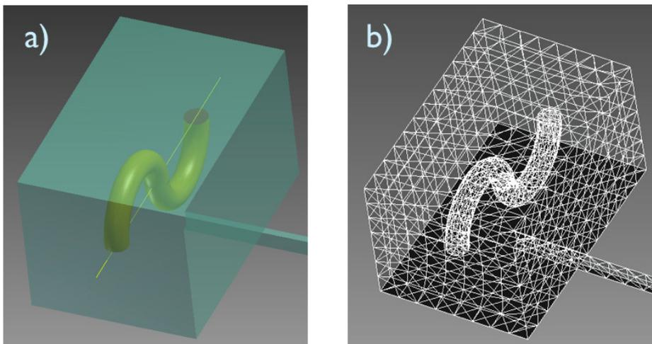
**Figure 1.** A geometry defined in CAD (a) can be transported to Geant as a mesh of triangles using STL format (b).
