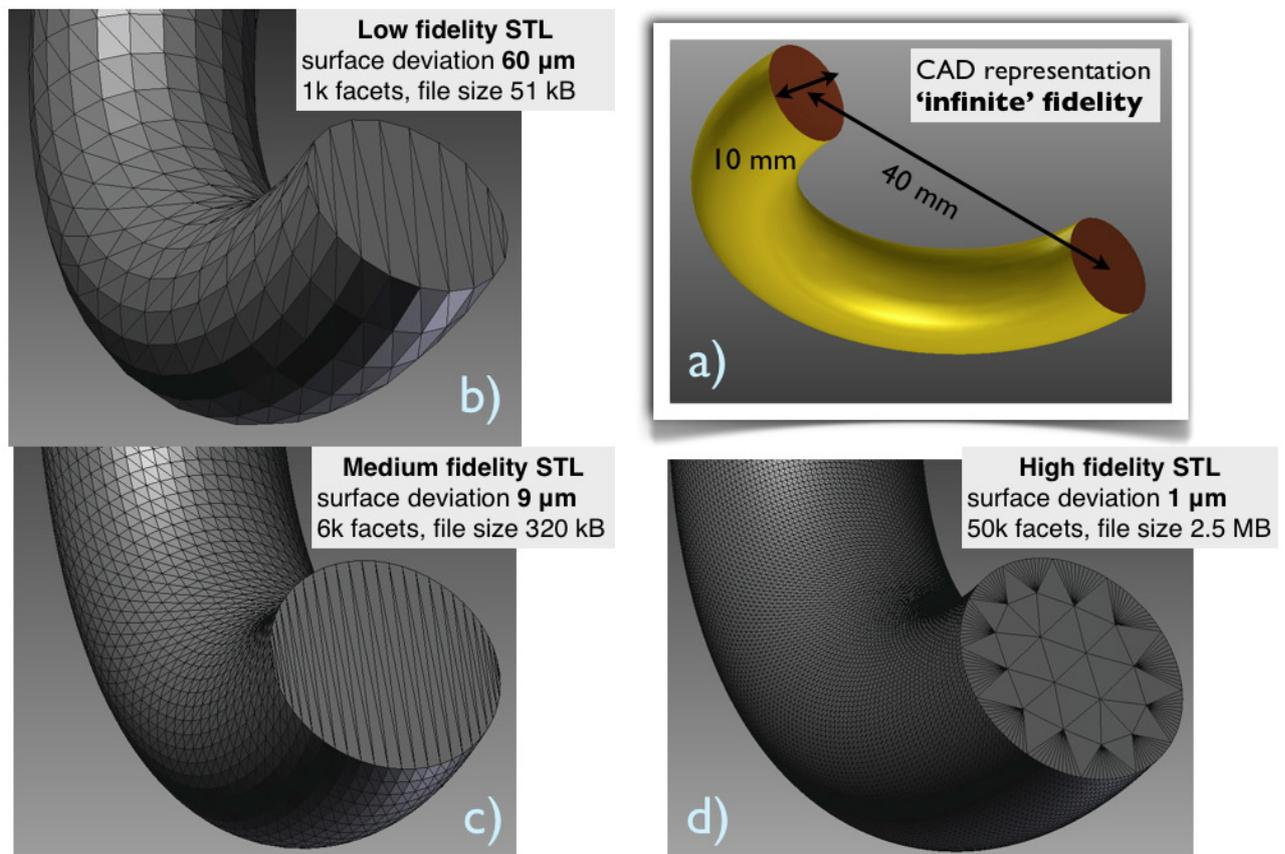
**Figure 3.** The STL file size and number of facets strongly depend on the required fidelity. (a) is ideal CAD geometry, (b)-(d) show consequences of decreasing maximal deviation of STL from  $60\mu$  to  $1\mu$ .
