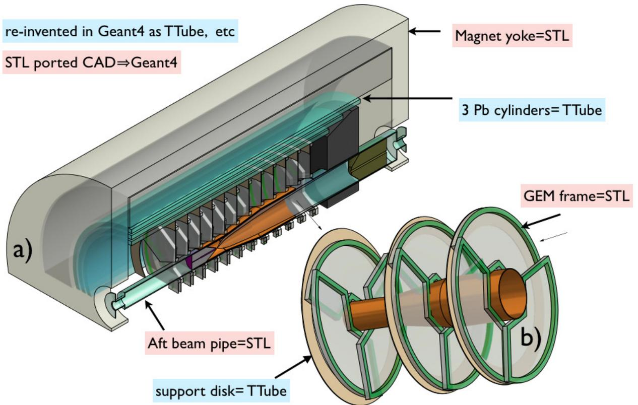
**Figure 5.** Illustration of a complex geometry of a detector (a). Only more complex parts (b) are exported from CAD to Geant using STL file format.
