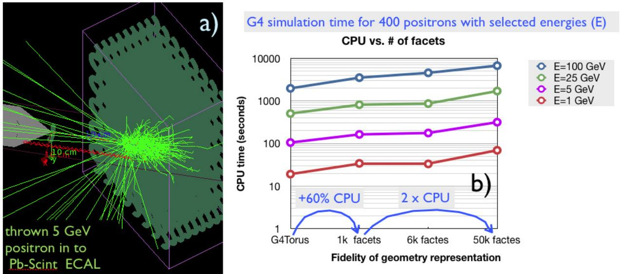
**Figure 4.** (a) The Geant model of a plastic-lead EM calorimeter used for (b) evaluation of the CPU cost of simulations. Different STL resolutions are labeled on the x-axis, results for different energies of the incident particle are shown with different colors.
