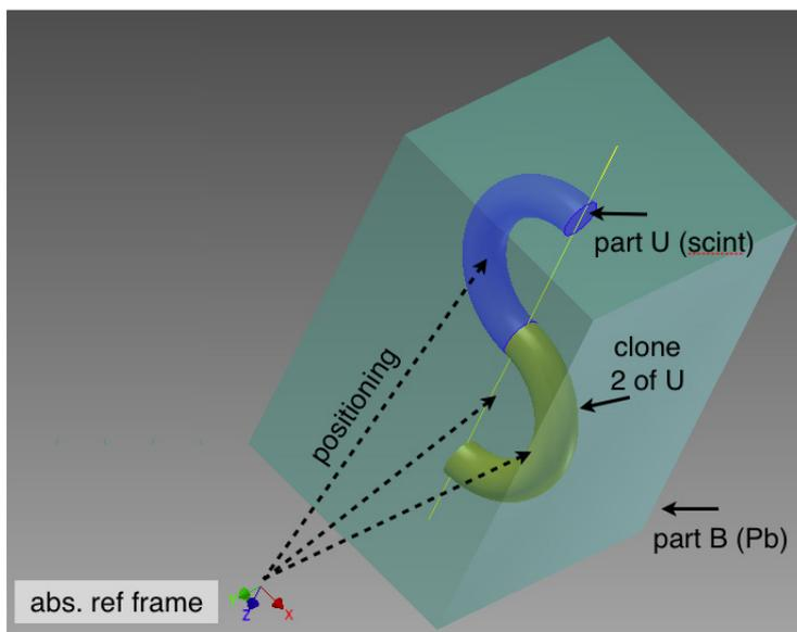
**Figure 2.** Building a complex object (S-shape) in Geant by replicating and translating the elementary object (U-shape).
