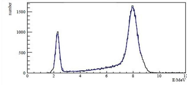
Fig.3.: Energy distribution of the Am-C neutron events.
