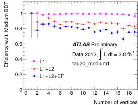
**Figure 16.** Tau trigger efficiency with respect to offline identified tau candidates as a function of number of vertices measured in 2012 data [8].
