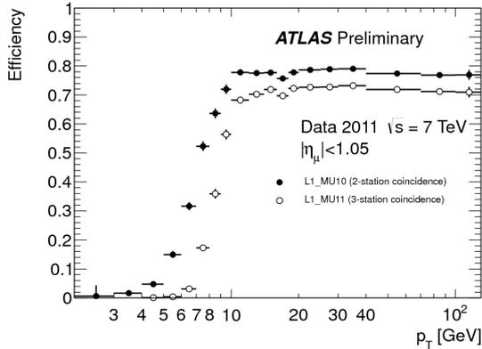
**Figure 5.** L1 trigger efficiency with respect to isolated offline combined muons for the barrel region as a function of the offline combined muon transverse momentum. The efficiencies include geometric acceptance of the detectors [5].
