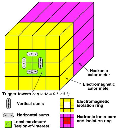
**Figure 11.** Building blocks of the tau algorithm with the sums to be compared to programmable thresholds.
