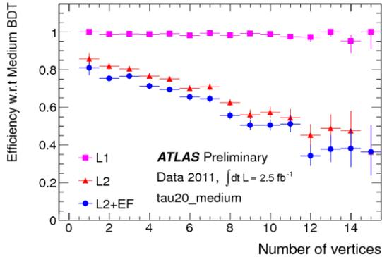
**Figure 15.** Tau trigger efficiency with respect to offline identified tau candidates as a function of number of vertices measured in 2011 data [8].
