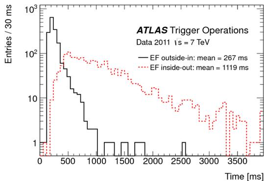
**Figure 9.** Execution times of the EF OutsideIn (solid line) and InsideOut (dashed line) muon triggers [5].
