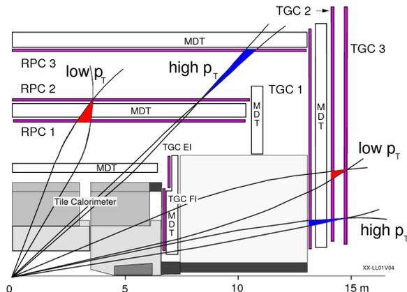
**Figure 3.** Quarter-section of the muon system in the  $z - y$  plane [5].
