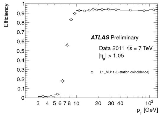
**Figure 6.** L1 trigger efficiency with respect to isolated offline combined muons for the endcap regions as a function of the offline combined muon transverse momentum. The efficiencies include geometric acceptance of the detectors [5].
