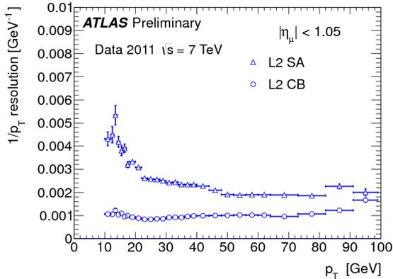
**Figure 7.** Resolution of the inverse  $p_T$  track parameter of the L2 SA and L2 CB algorithms as a function of the offline muon  $p_T$  in the barrel region [5].
