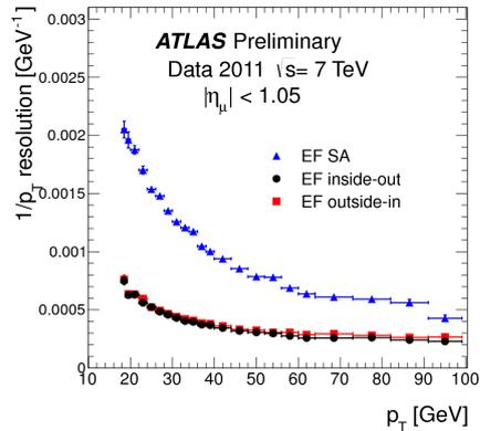
**Figure 8.** Resolution of the inverse  $p_T$  track parameter of the EF SA and EF InsideOut and OutsideIn CB algorithms as a function of the offline muon  $p_T$  in the barrel region [5].
