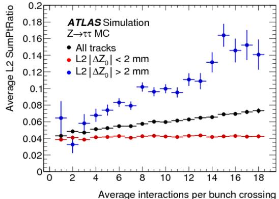
**Figure 14.** Average L2 SumPtRatio as a function of the average number of interactions per bunch crossing for different track selections [8].
