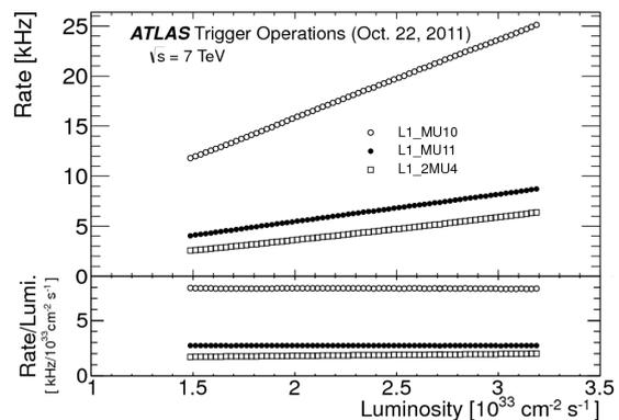
**Figure 4.** Level 1 muon trigger rates versus the instantaneous luminosity in 2011 [5].
