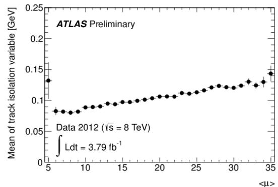
**Figure 10.** Track isolation variable as a function of number of interactions per bunch crossing [6].
