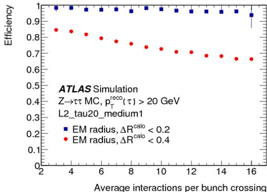
**Figure 13.** L2 tau trigger efficiencies using the L2 EM radius calculated in cones of  $\Delta R < 0.2$  and  $0.4$  as a function of the average number of interactions per bunch crossing [8].
