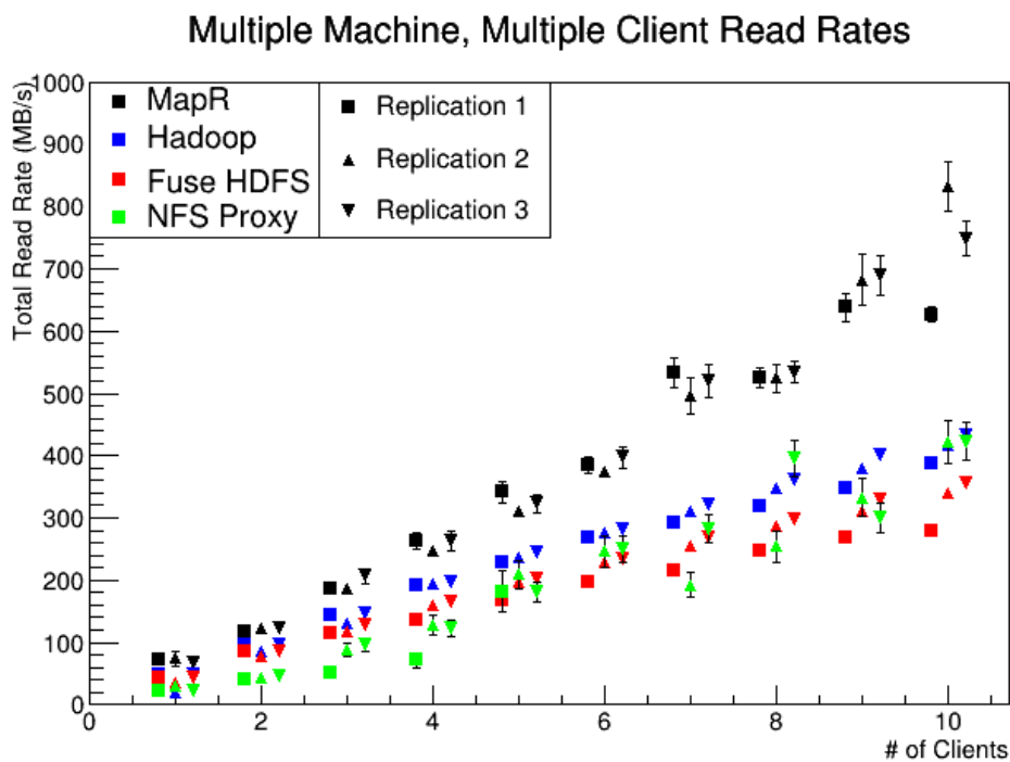
Figure 2. The scaling of read rates as a function of number of clients for a single 1 GB file.
